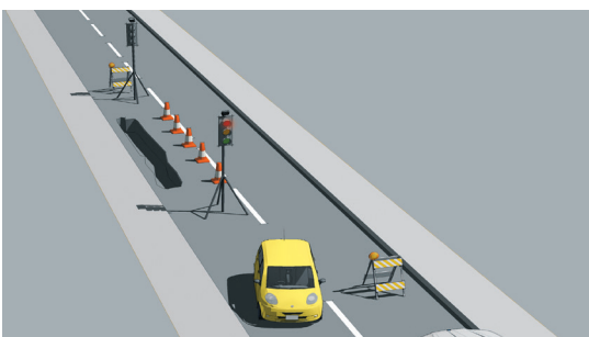
Temporary traffic control
