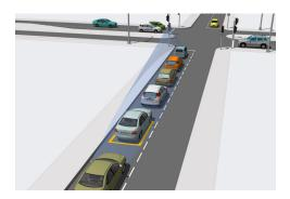
The 318's accurate virtual-loop technology, with speed discrimination & stationary detection can emulate two inductive-loops up to a range of up to 150 metres, or lane-specific detection up to 40 metres with one 318 per lane. In traffic control applications, the 318 tracks up to 12 targets and 'reports' when virtual-loops are triggered. The 318 can make loops 'smart' as well - for example, to prioritise buses over cars at bus-gates.
