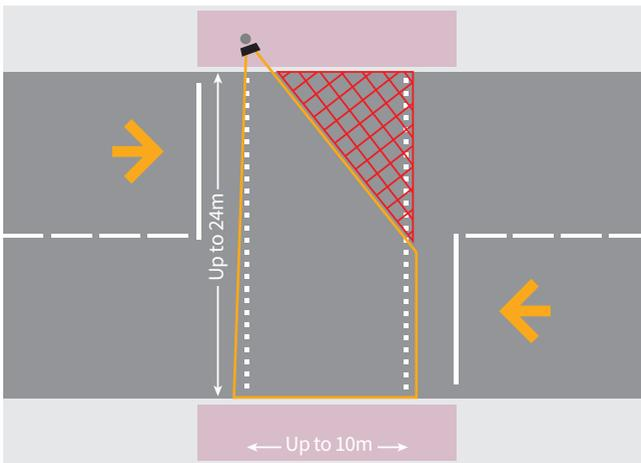
Two detectors installed together cover described dead spots.
