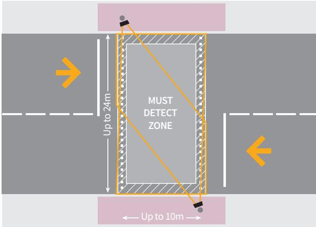
**Please note:** The radars have a 'may detect zone' surrounding the must detect zone to avoid false detections from the kerb edge and vehicles encroaching on the stop line. The AGD326 also has a  $\pm 1$ meter accuracy due to the calibration encoded on the detector. This is more noticeable on the extremities of the radars range
