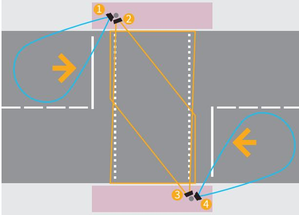
The devices numbered 1 to 4 are representative of radar traffic detectors, these can be either AGD306, AGD326, AGD316 or AGD318.
