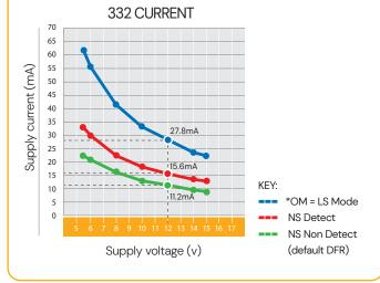
The AGD332 radar has taken the powerful feature rich experience from the low power AGD331. Using the latest power saving technology, the radar's design is a unique pulsed, frequency modulated transceiver linked to a 32bit ARM Cortex M4 processor. This helps deliver market leading radar performance while maintaining extremely low power usage.
