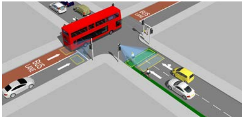
Mount on the side of the road with the lowest number of large vehicles (bus lanes/HGV routes)
