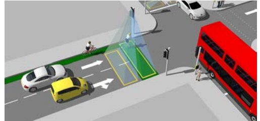
Mount on the side of the road closest to approaching cyclists for cycle refuge applications
