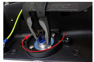
Loosen switch barrel using pipe pliers
