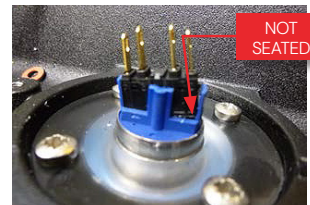
Micro switch located INCORRECTLY
