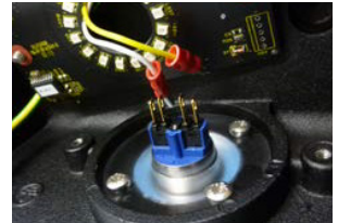
Remove Halo pcb and terminals
